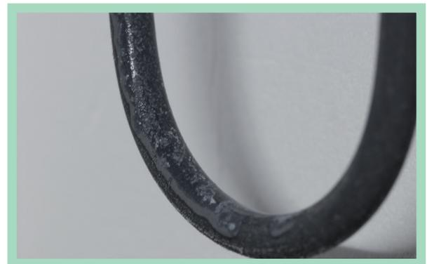
Fig. 4: Crystals of quartz crystals lead to contamination
