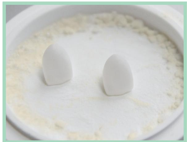
Fig. 2: Result after sintering with **Nacera<sup>®</sup> Clean LT** application
