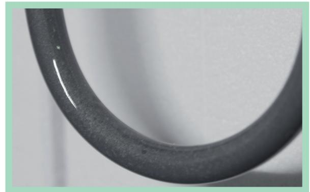
Fig. 3: Heating element with intact, vitreous protective coating
